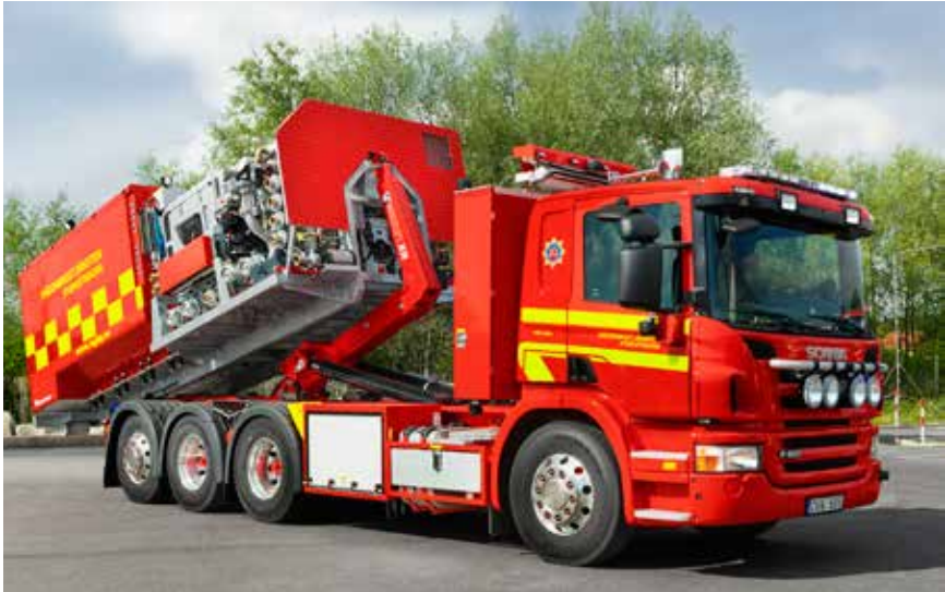
Rosenbauer assembles individual roll-off containers for every fire department. The substructure forms an L-base frame in accordance with the valid DIN standards.
