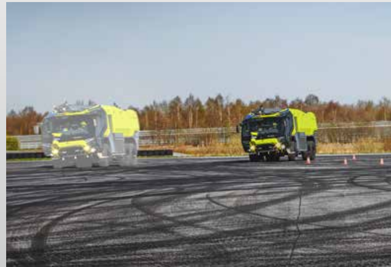
Driving through corners at high speed without / with RSC
