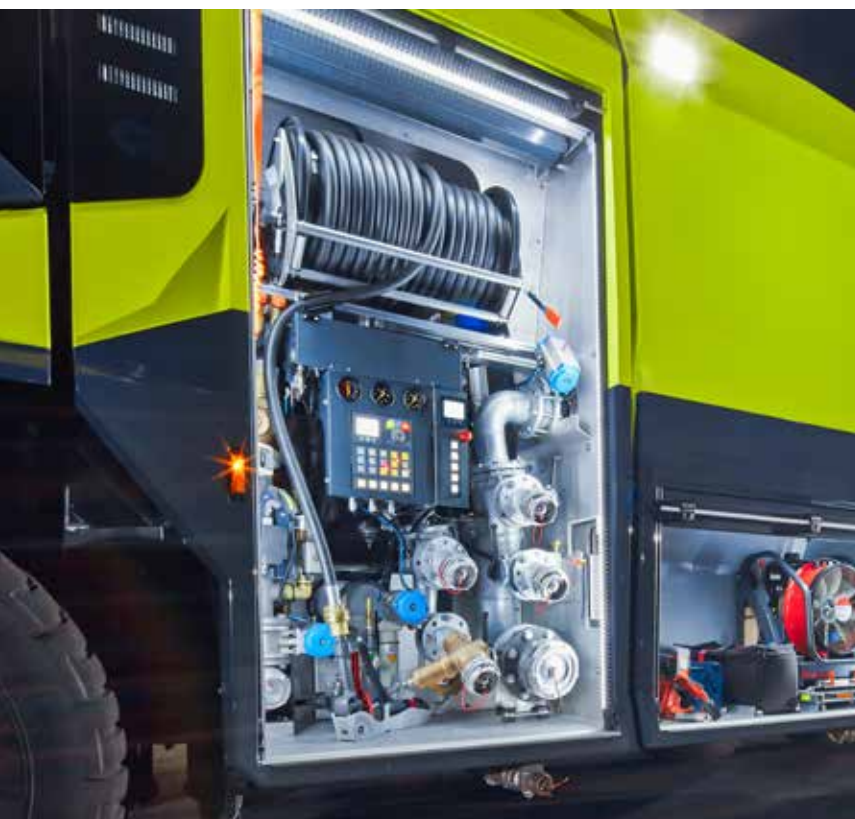
Pump compartment illumination
