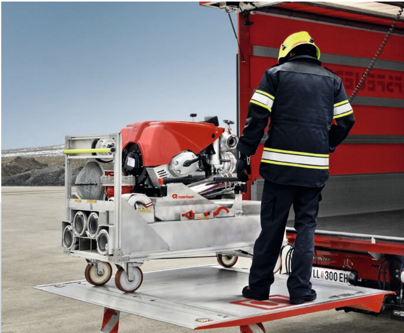
Lifting platform for simple loading and unloading of equipment weighing up to 1,000 kg.
